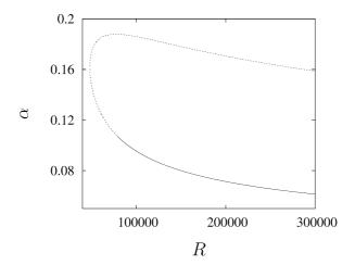
Fig. 2. Sign distribution of  $a_1$  along the linear stability neutral curve. The continuous and dashed lines correspond to supercritical and subcritical instability respectively.
